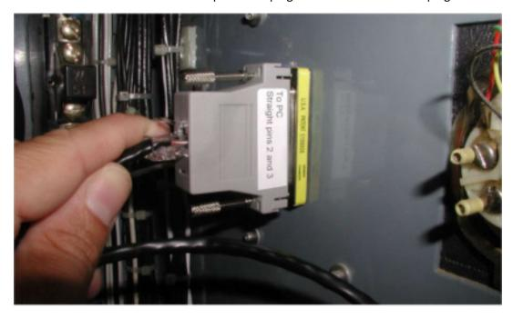
Mount the included DB25 female-female plug to the cabinet. Then the DB25 to RJ45 connector labeled "To PC" can be plugged into back of female-female plug on the cabinet panel.
