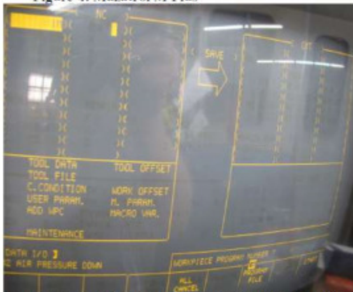
Figure 6: Save or Load programs on a Mazatrol M Plus control
