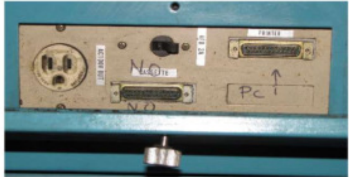
Figure 9: Mazatrol will probably have two DB25 female connectors, the one labeled Cassette must be used to save and load Mazatrol conversational programs. Sometimes the port is label with a picture of a cassette tape. The other DB25 is used only for EIA G code programs
