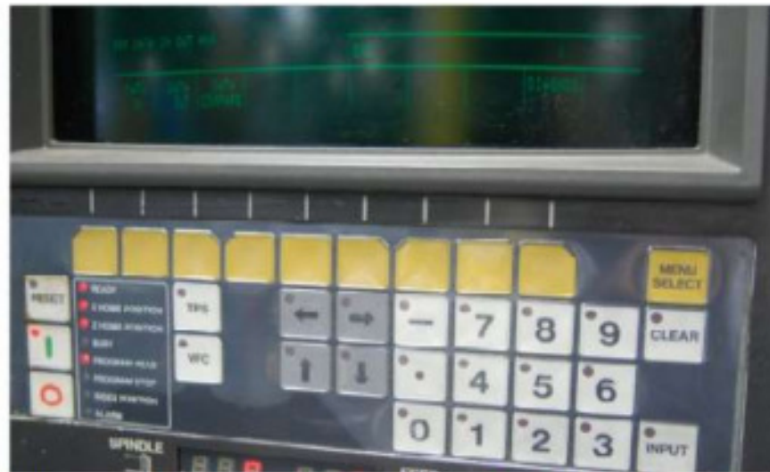
Figure 3: DATA IN and DATA OUT soft keys, INPUT hard key and the display showing END indicating the completion of DATA IN
