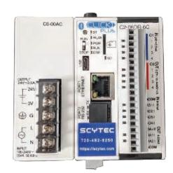
The Status Relay Controller (SRC) is a low-cost hardware device that comes programmed and ready to work with Scytec DataXchange. The SRC can be connected to a wired or wireless Ethernet network and is capable of monitoring digital and analog signals with built-in functionality around shop floor equipment. The SRC is available in two configurations, the SRC Standard and the SRC Extended.
