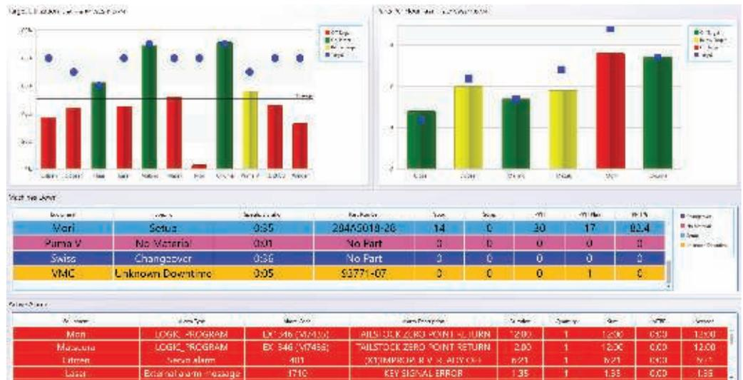
A dashboard configured to show utilization against targets, parts per hour against targets, machines currently in a downtime, and machine alarm detail.
